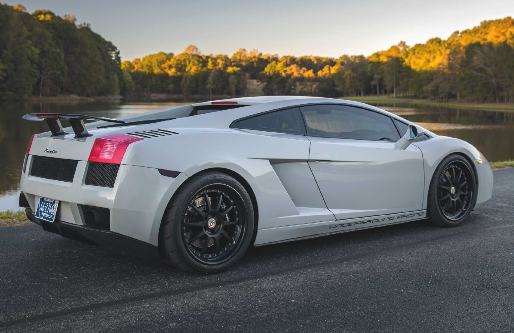
Above Wheels are HRE C103 forged three-piece split-rims, their 19-inch diameter chosen to offer the ideal mix of acceleration and top-end. HRE competition-spec wheels were chosen because they're incredibly light and strong
