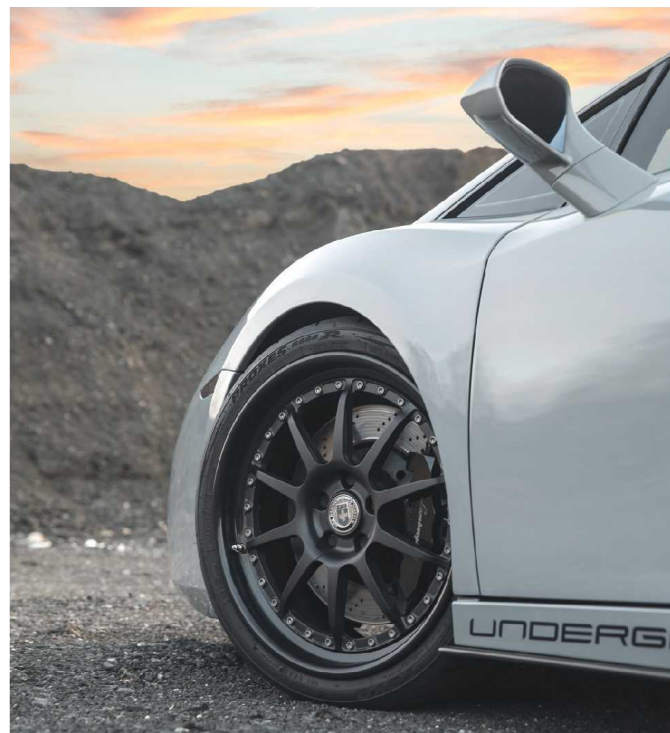
Above Wheels are HRE C103 forged three-piece split-rims, their 19-inch diameter chosen to offer the ideal mix of acceleration and top-end. HRE competition-spec wheels were chosen because they're incredibly light and strong
