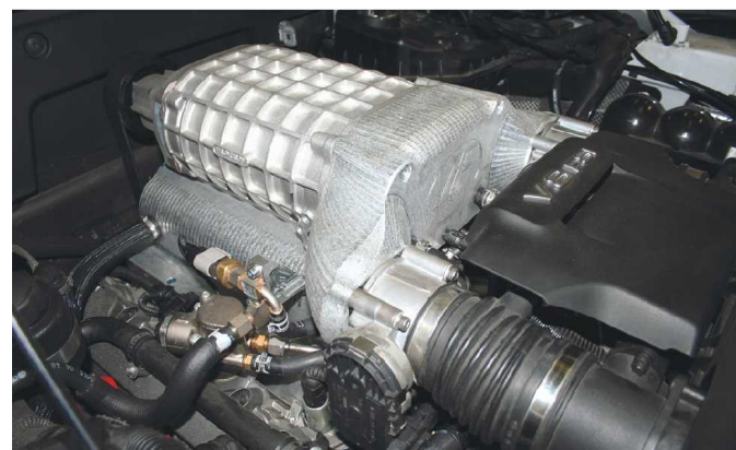
Below left VF Engineering's positive displacement R8 supercharger setup
